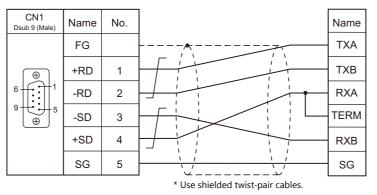
For 1 : 1 connection: Terminating resistance:  $120\Omega$  with RXA and TERM short-circuited
