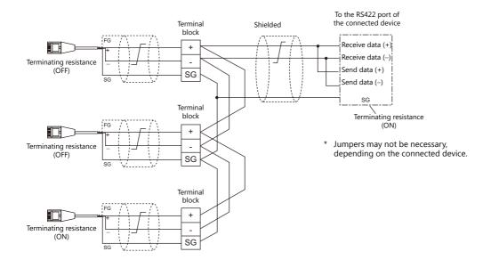
This shows the situation when a multi-link connection is made at MJ1 or MJ2.
