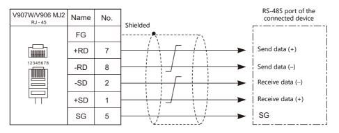
• If noise disturbs communications, connect a shielded cable to both the V9 series and the connected device.
