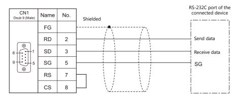
• If noise disturbs communications, establish connections between SD and SG and between RD and SG as pairs respectively, and connect a shielded cable to both the V9 series and the connected device.
