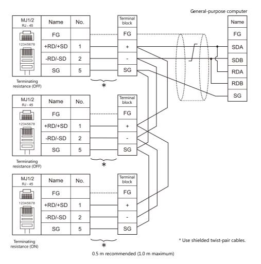
\* Set the slide switch for signal level selection to RS-232C/485 position (upper) when using the MJ2 port of V907W or V906. For details, refer to "1.2.2 MJ1/MJ2" (page 1-6).
