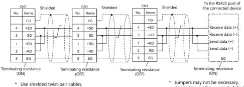
Jumpers may not be necessary, depending on the connected device.
