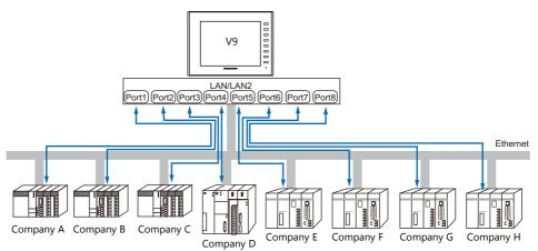
• When there are two or more PLCs of the same model, the V9 series is allowed to carry out 1 : n communication via one single port.
