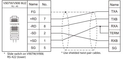
For 1 : 1 connection: Terminating resistance:  $120\Omega$  with RXA and TERM short-circuited
