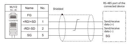
• If noise disturbs communications, connect a shielded cable to both the V9 series and the connected device.
