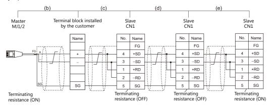
As a measure against noise, connect the frame ground terminal of each V9 series at one side only. The frame ground of V6-MLT must be connected to the V9 series
