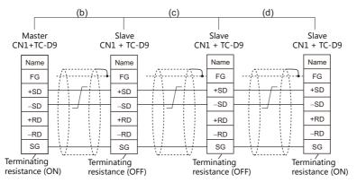
\* As a measure against noise, connect the frame ground terminal of each V9 series at one side only.
