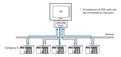
• If multiple V9 units are connected to one single PLC, the maximum permissible number of these units depends on the PLC specifications. Refer to the PLC manual issued by the manufacturer.
