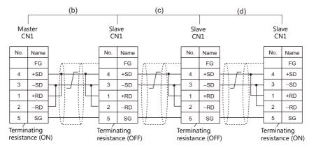
\* As a measure against noise, connect the frame ground terminal of each V9 series at one side only.
