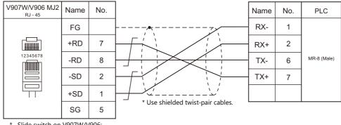
\* Slide switch on V907W/V906: RS-422 (lower)
