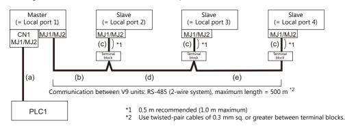
Connecting the MJ1/MJ2 of the master to the MJ1/MJ2 ports of the slaves
