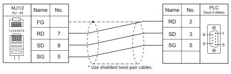
The send/receive wires are crossed inside the device.
