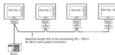
You can make settings for multi-link at the PLC1. Therefore, multi-link connection is not possible concurrently with a network connection that uses a "CUR-xx" communication interface unit. A physical port is selectable from CN1, MJ1, and MJ2.
