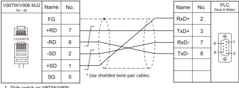
Slide switch on V907W/V906: RS-422 (lower)
